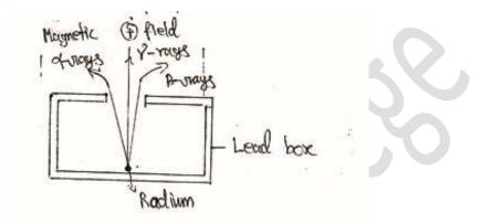
In the above diagram radium is kept in the lead box  $\alpha$ ,  $\beta$  and  $\gamma$  rays are coming out from the radium. The magnetic fields is applied to separate the  $\alpha$ ,  $\beta$  and  $\gamma$  rays
