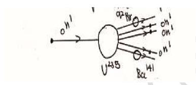
In the above diagram, the projective is the slow neutron, target nucleus is uranium, product nuclei are  $\beta$  and the outgoing particle are neutrons.
