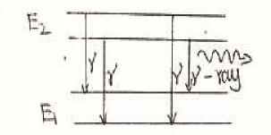
In the above diagram, there are two nuclear levels. The energy of upper level is  $E_2$ . The energy of lower level is  $E_1$ .  $\gamma$  rays are emitted in the diagram.
